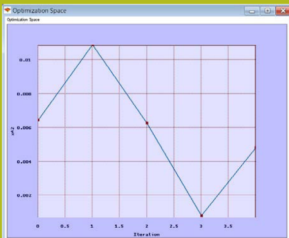
Fig 6 (a). Calculated values of \chi^2 are gradually decreasing during iterations 0 - 4
